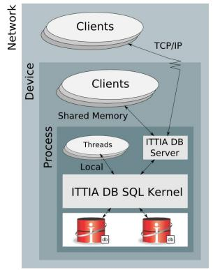
process through shared memory or TCP/IP. Regardless of how many connections there are or how they are made, each database file uses only one page cache.
